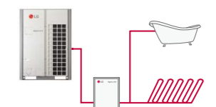
Hot water+ Radiant heating
